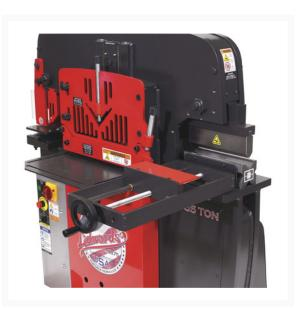
The Press Brake Back Gauge allows users to easily set up repeatable bends. Speed up your production with this simple to use positive stop gauge. Compatible with all Edwards Ironworkers and Shop Presses.
